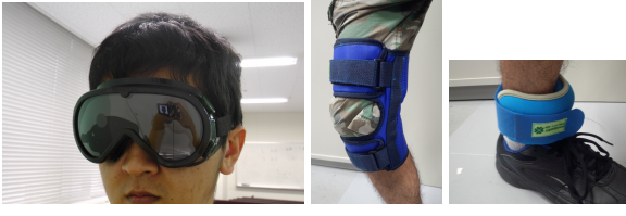
Fig. 16 Tools for simulating the physical situation of the elderly. The left: the goggle simulates a visual deficit. The center: the band limits the movement of the knee joint. The right: the 1kg load simulates the decrease of the physical strength.
